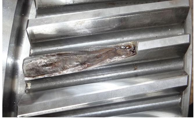
Gear suffering tooth breakage
