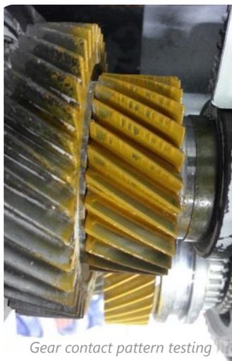
*Gear contact pattern testing*
